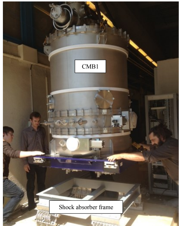
Figure 8: CMB1 “kiss landing” operation on the shock absorber frame.
