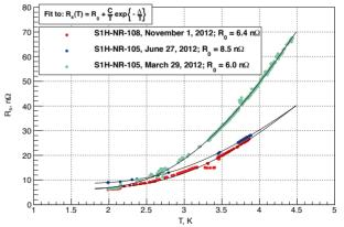
Figure 4: Measurement of surface resistance vs temperature.
