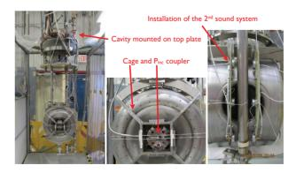
Figure 1: SSR1 cavity attached to the VTS top plate.
