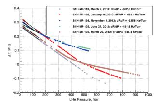
Figure 3: Measurement of the resonance frequency shift vs LHe bath pressure during cool-down from 4.4 K to 2 K.
