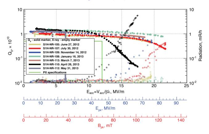
Figure 6: Summary of results of SSR1 cavity tests at 2K.
