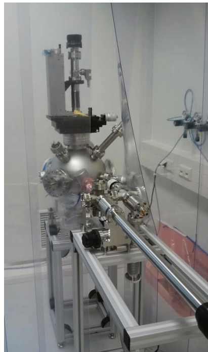
Figure 7: Photograph of the new preparation system for GaAs photocathodes.
