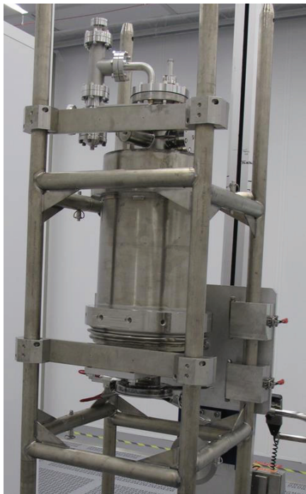
Figure 5: Photograph of SRF gun cavity with He tank before the vertical test.
