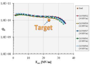
Figure 8: Vertical test result of some cavities.
