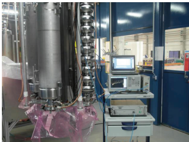
Figure 4: An XFEL cavity in the insert – RF measurement (room temperature).
