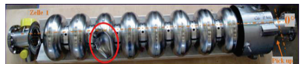
Figure 6: Fine grain cavity after pressure test with 31bar with dent in cell three.
