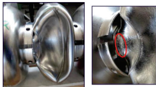
Figure 7: Deformation and breakage at iris of cell three.
