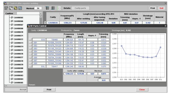
Figure 2: RF quality control panels for Acceptance Level 1.
