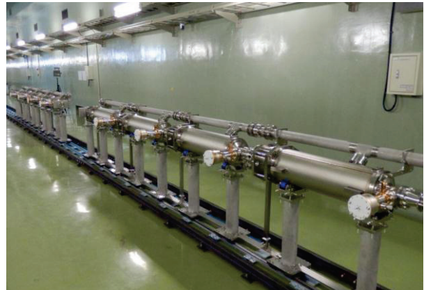
Figure 2: STF cavities with jackets governing high pressure gas safety law in Japan.
