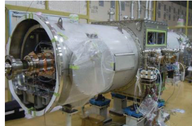
Figure 9: Cryomodule for c-ERL main linac
