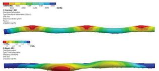
Figure 12: Structural analysis of the HGRP showing vertical displacement and the lowest mechanical eigenmode.
