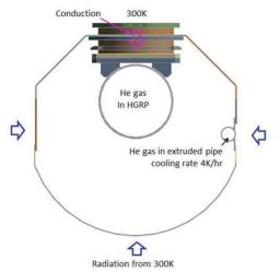
Figure 13: Asymmetric cooling of the 40 K thermal Shields.
