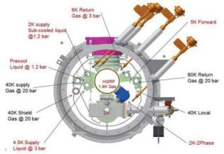
Figure 11: Cross-section of the module.
