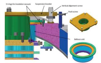
Figure 6: Post alignment components.
