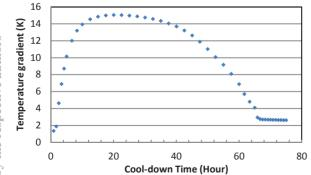
Figure 15: Temperature gradient on 40 K shield as a function of time during cool-down.
