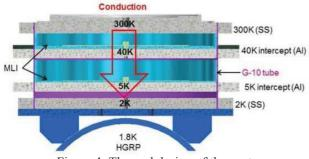
Figure 4: Thermal design of the post.
