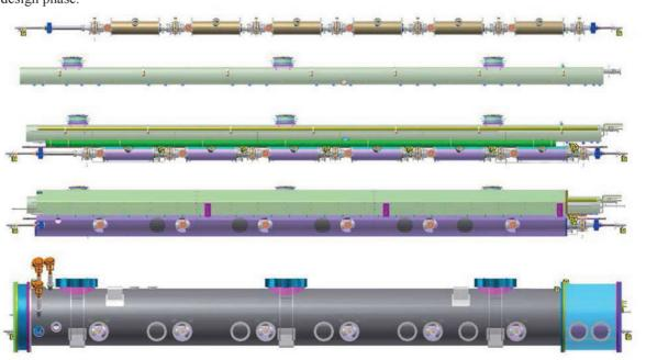
Figure 20: MLC prototype assembly sequence.
