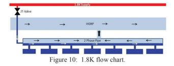
above the critical point for liquid helium (around 3 bar), where helium gas conveniently has an increased heat capacity. The choice of temperature rise between supply and return is a compromise between reducing the mass flow of gas through the refrigeration system to improve refrigeration efficiency and keeping the outlet temperature low enough to not degrade superconducting properties of the cavities.
