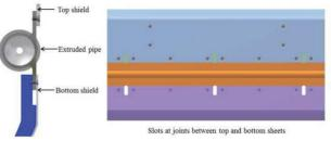
Figure 8: Joints between top and bottom sheets.
