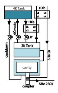
Figure 2: Valve Box Flow diagram.
