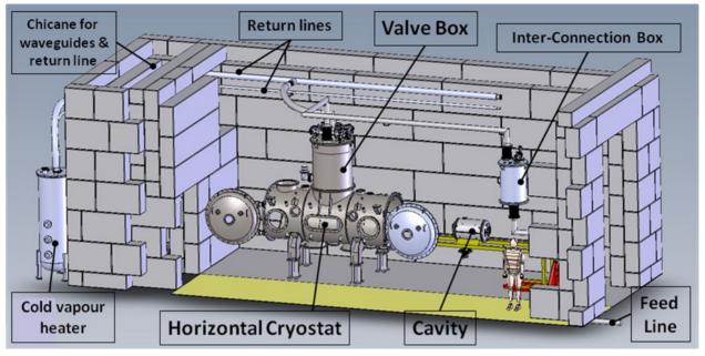
Figure 1: Layout of the FREIA bunker.
