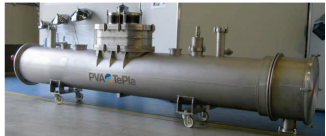
Figure 2: Photo of the new cryostat module. The stadium shaped tower section in the middle houses the WR-284 transition lines.
