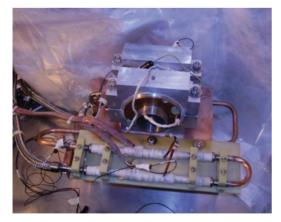
Figure 2: Test coil and LHe heat sink.
