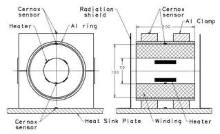
Figure 1: Test magnet and embedded instrumentation.
