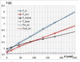
Figure 4: Temperatures in the test magnet at different settings of the heater.
