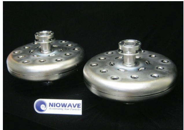
Figure 5: Photograph of the 2.1 GHz PBG cavities with elliptical rods ready to be tested.
