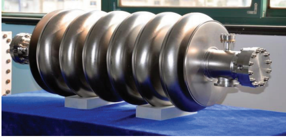
Figure 4: Prototype of the NJU medium-beta SRF cavity.
