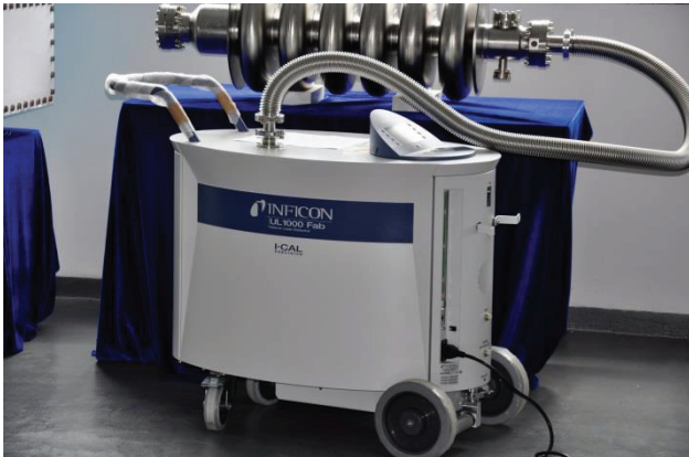
Figure 5: Vacuum test for the NJU medium-beta SRF cavity.
