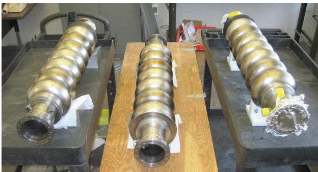
Figure 1: Three ERL cavities built at Cornell to be installed into the prototype Main Linac Cryomodule (MLC).
