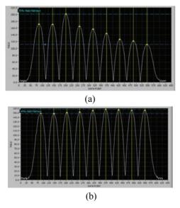
Figure 2: field flatness of PKU4. (a) before flatness tuning (b) after flatness tuning.
