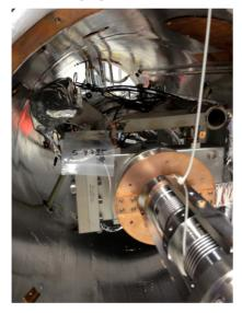
Figure 4: CC-1 internal view with new cavity inserted.
