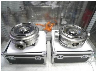
Figure 7: Two bare Spoke012 prototype cavities fabricated in November 2012.
