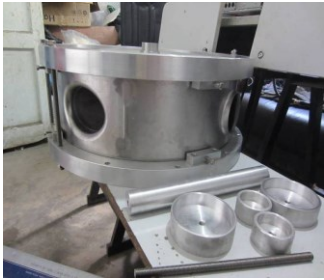
Figure 6: A frock clamp for Spoke012 tuning.
