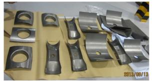
Figure 7: Components after deep-drawing.
