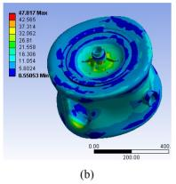
Figure 6: Distribution of deformation (a) and stress (b).
