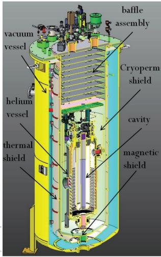
Figure 3: 56 MHz cavity assembly in the BNL's LVTF dewar.
