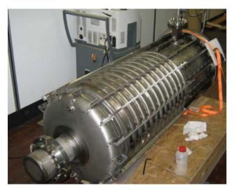
Figure 2: 56 MHz SRF cavity without helium vessel.
