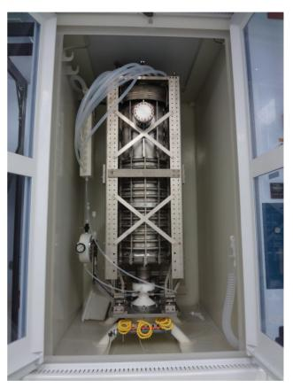
Figure 4: Cavity set up for BCP in the clean room.
