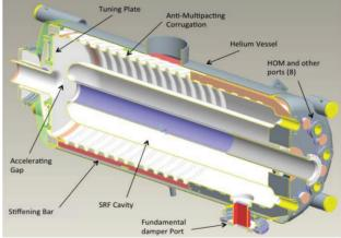
Figure 1: Top: Layout of ports for the 56 MHz SRF cavity for RHIC; Bottom: Cross-sectional view of the cavity with helium vessel.
