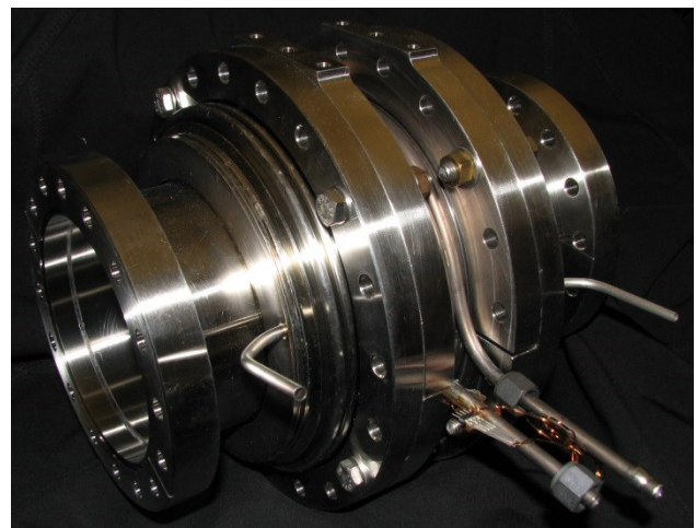
Figure 1: Cross-section of the HOM absorber currently being installed in the Horizontal Test Cryomodule (HTC). The absorbing material is SiC brazed to tungsten.
