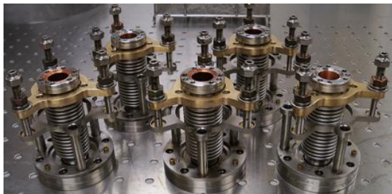
Figure 7: Processed FPC assemblies in ISO 5 cleanroom.
