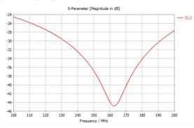
Figure 3: S11 as a function of frequency.
