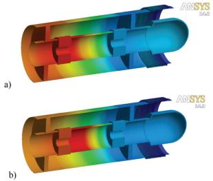
Figure 6: Temperature maps of a coupler operating at resonant frequency (a) and off resonance (b) (red -356 K, blue -2 K).
