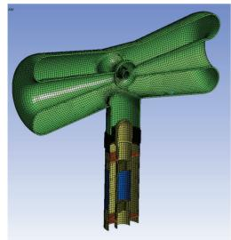
Figure 4: Power coupler connected to the HWR.
