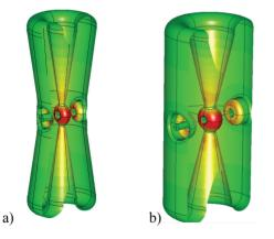
Figure 1: Electric field distribution in  $\beta$ =0.12 (a) and  $\beta$ =0.24 (b) cavities.
