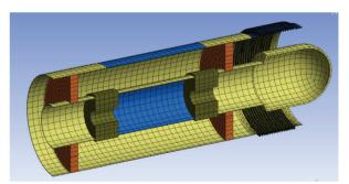
Figure 2: RF power coupler design after the optimization.
