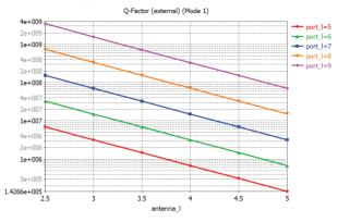
Figure 5: External Q-factor as function of the antenna's length for different RF port dimensions.
