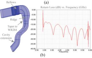
Figure 4: HOM waveguide assembly: (a) CAD geometry and (b) RF simulation model with return loss.
