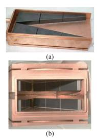
Figure 2: HOM damper assemblies: (a) copper damper half with soldered SiC tiles and (b) ebeam welded prototype damper assembly.
