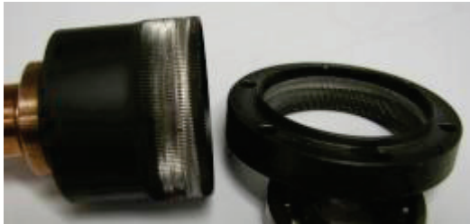
Figure 7: Harmonics drive gear failure.
