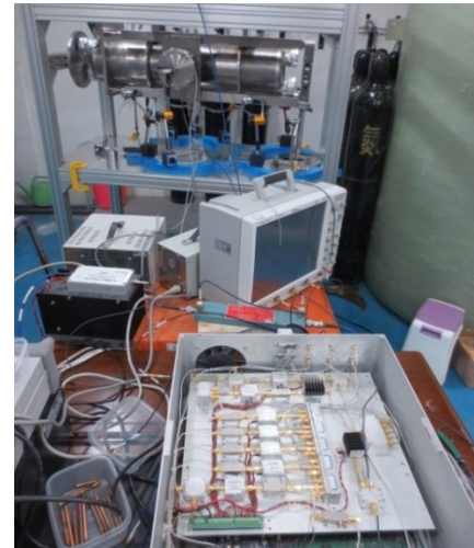
Figure 3: The experimental setup for tuning with Low Level RF system.
