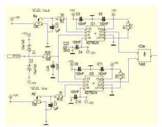
Figure 4: Klystron focusing coil electronic, this scheme is the same for the 2 PS (bucking coil and solenoid) for voltage and current.
