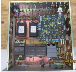
Figure 3: Supratech klystron compact interlock system.
