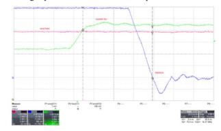
Figure 5: New interlock system response time, less than 80ns to switch off the klystron HV pulse (gray : up threshold, green : focusing coil current, HV pulse enable signal).
