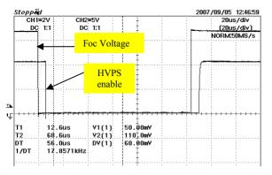
Figure 2: NI-PXI FPGA Response time to focusing coil default is about 10µs.
