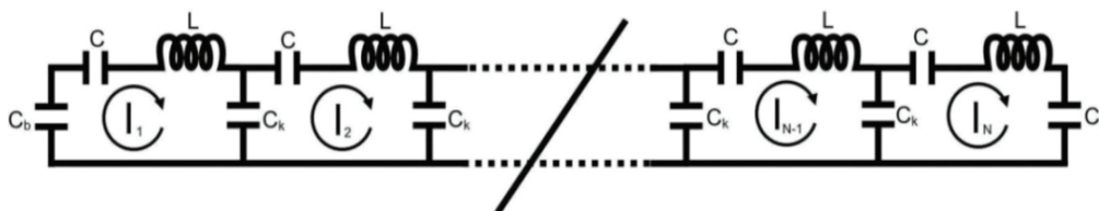
Figure 3: RLC cavity and beam tubes equivalent circuit.
