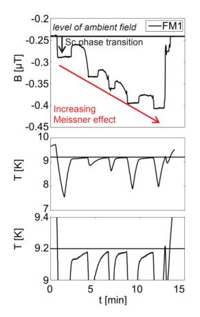
Figure 5: Behavior of trapped flux (FM1) and temperature upon heating in ambient field (0.3  $\mu$ T in FM1 direction, 3  $\mu$ T in total).
