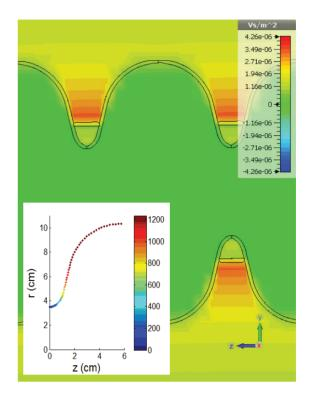
Figure 3: Simulation of the magnetic field distribution around a TESLA cavity that carries a current of 1A. Insert: Simulation of the surface H-field distribution of the accelerating  $\pi$ -mode (courtesy Axel Neumann).
