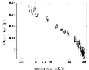
Figure 4: Expelled flux measured by FM1 versus cooling rate in the model system.  $B_{nc}$  during the measurement was 0.3  $\mu$ T in FM1 direction and 3  $\mu$ T in total.
