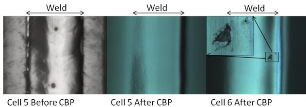
Figure 5: Internal inspection of NR1 before and after mirror like finish CBP. Moving from left to right dual eye defect in cell 5, the same location after 20  $\mu\text{m}$  EP (no effect) and 4 step CBP, and new defect at the edge of the equator in cell 6 not see before CBP.
