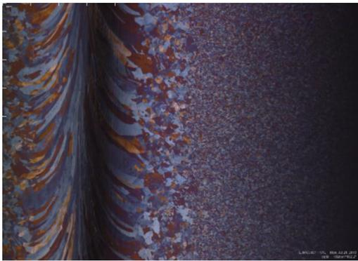
Figure 7: Internal optical inspection of the weld area on a 1.3 GHz XMP copper cavity after cleaning but without chemistry. Image size approximately 1.5 cm×1.5 cm.
