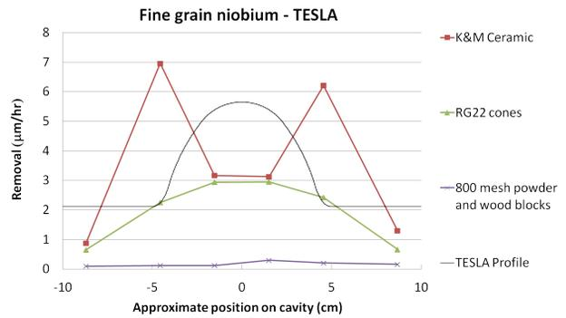
Figure 4: CBP removal rate vs. position for different media types for TE1G003 - fine grain TESLA shaped 1.3 GHz for the first three CBP steps. The markers are the approximate measurement location on the cavity with the connecting lines as a guide to the eye as is the TESLA profile in thin black [8].
