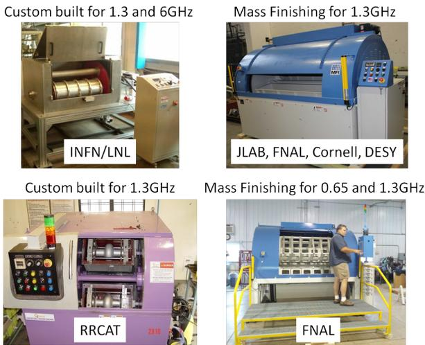
Figure 1: CBP machines from around the world. Designed elliptical cavity frequency, manufacturer if built outside the host laboratory (custom if built inside the lab), and lab location is shown in the text for each machine.
