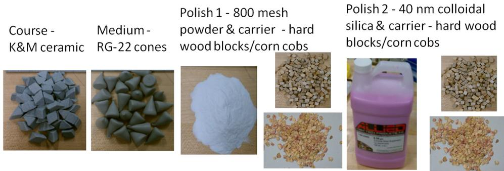
Figure 3: Standard CBP recipe used by various labs. The run time varies between labs depending on the application. Course (6 hours or longer), medium (12 to 30 hours), polish 1 (20 to 40 hours), and polish 2 (40 to 300 hours).
