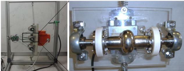
Figure 9: Image of resonant vibration system at INFN/LNL designed for 6GHz cavities.
