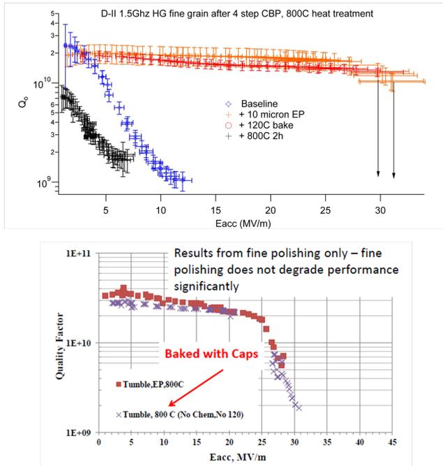
Figure 8: Top: Test results from D-II at JLab, the baseline results are from CBP and heat treatment with no chemistry. Additional light chemistry and low temperature bake improved the cavity. Final heat treatment with no chemistry showed a strong Q slope attributed to furnace contamination. Bottom: Test results from Large grain 1.3 GHz cavity showing the final CBP step does not degrade cavity performance.
