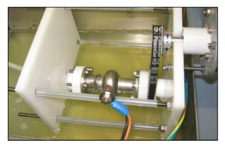
Figure 10: The new system for the electropolishing half of cavity.
