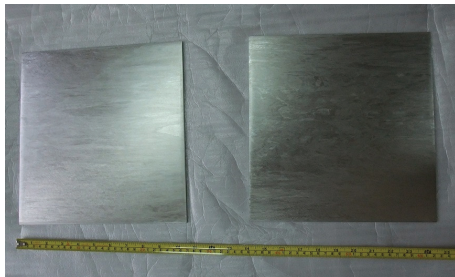
Figure 7: Nb sheets doped with Sc, 265mm \times 265mm \times 2.8mm .
