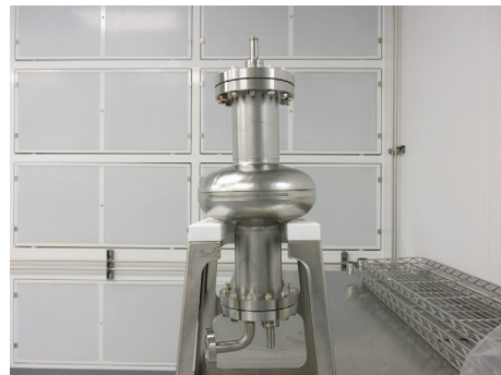
Figure 9: 1.3 GHz Tesla-type single-cell cavity. The equator welds was done in JLab.
