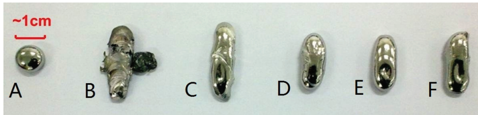
Figure 1: Nb samples from OTIC. Sample A was pure Nb. Sample B failed to melt. Samples C to F were doped with different proportions of Sc.
