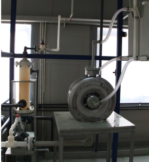
Figure 3 : Pipes connection of spoke cavity.
