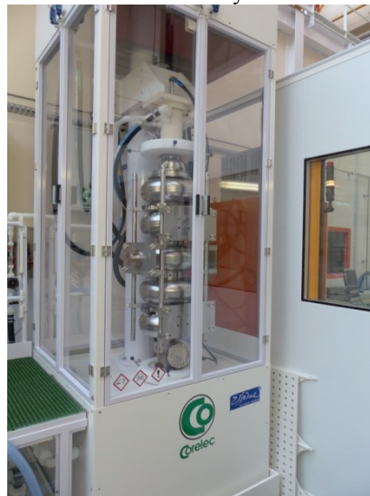
Figure 1: 5-cell SPL cavity during VEP treatment.
