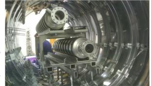
Figure 3: 800 C UHV oven loaded with two XFEL serial cavities.
