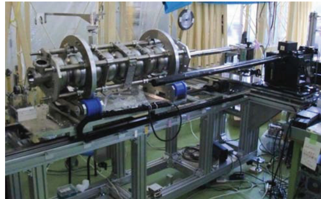
Figure 1: Combined cavity camera and local grinder system. The cylinders can be switched for a cavity in inspect and repair cycles.
