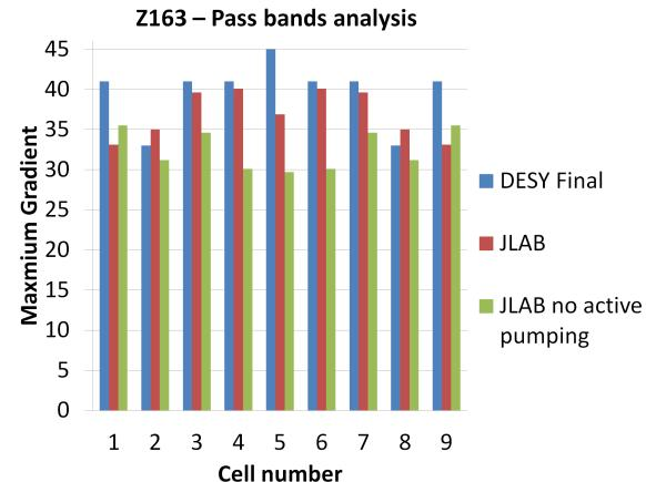
Figure 1: Compiled RF pass band analysis for three tests of Z163. Blue: final test at DESY  $\pi$  mode quench cell 8, Red: initial test at JLab  $\pi$  mode quench cell 9. Green: retest at JLab with no active pumping,  $\pi$  mode quench cell 5.
