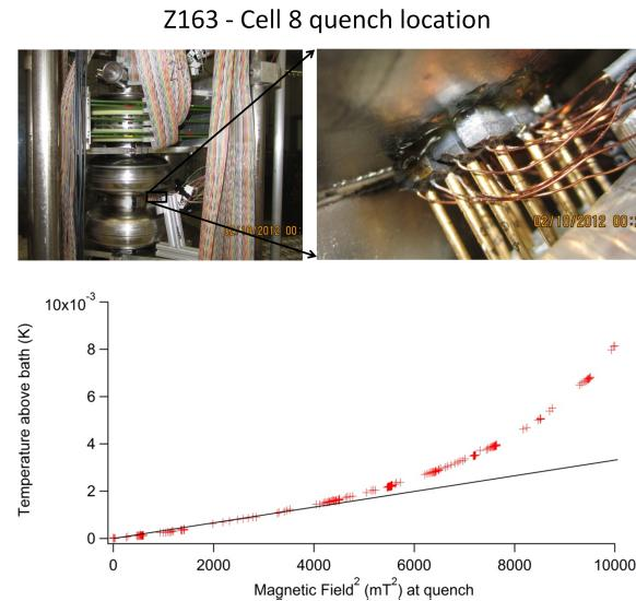
Figure 3: Quench location for cell 8 in Z163. Top: picture of top half of cavity in test stand, the right picture is a zoom in of the left picture showing the 4x4 temperature mapping array location at the quench location found at DESY. Bottom: temperature vs. magnetic field squares field scaled to quench location for the highest preheating temperature thermometer in the array.)
