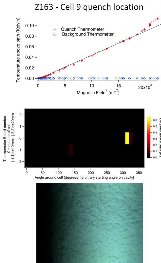
Figure 2: Quench location data for cell 9 in Z163, moving from top to bottom: temperature rise vs. magnetic field squared (field scaled to thermometer location field) for quench location thermometer in red, the background thermometer on the same board is shown in blue); unfolded temperature map from cell 9 after quench during cooling; inner surface optical inspection after disassembly showing no identifiable defect.
