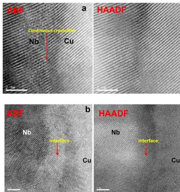
Figure 3: STEM micrographs for the Nb film/Cu substrate interface for films grown at (a) 360 °C (hetero-epitaxy) and (b) at 200 °C (fiber growth).
