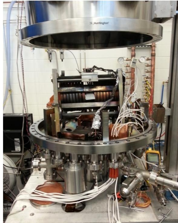
Figure 1: Inside the ECR sample coating system.
