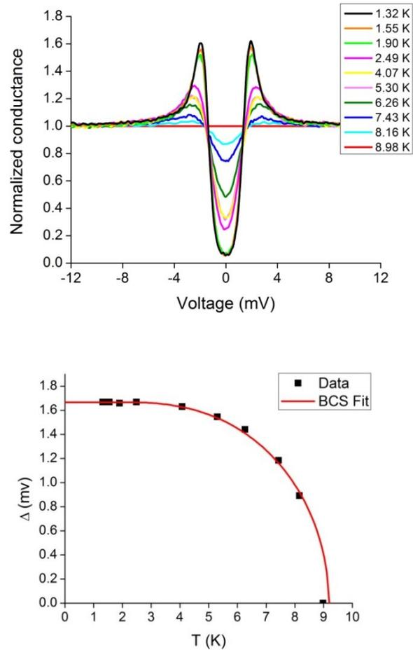
Figure 4: Superconducting gap measurement for a hetero-epitaxial polycrystalline Nb/Cu film (RRR=289).
