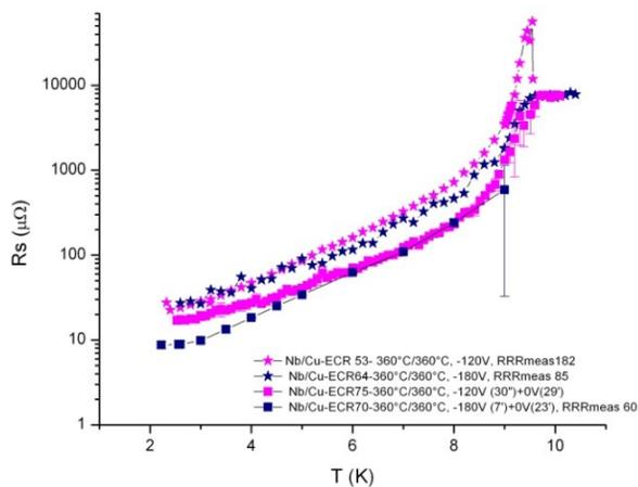
Figure 6: Surface resistance measurements for ECR Nb films coated with constant or varying ion energy during film growth.
