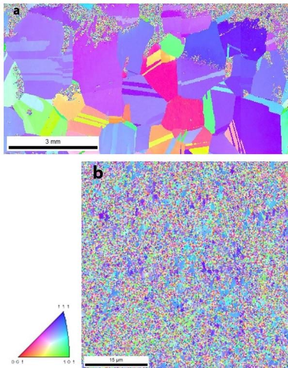
Figure 2: EBSD map for ECR films deposited on large grain Cu substrate with -120 V bias (184 eV) respectively at (a) 360 °C and (b) 200 °C (note the difference in scale).
