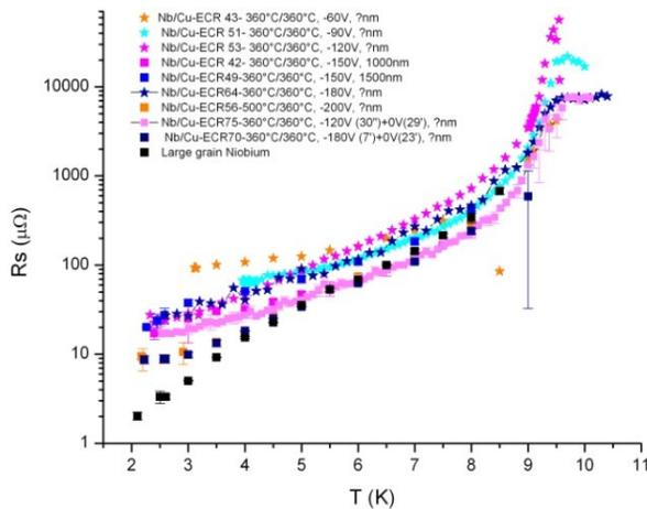
Figure 5: Surface resistance measurements for a series of ECR Nb films coated at various bias voltages and at 360 °C.
