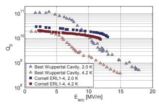
Figure 4: Q vs E curve from the new Cornell Nb<sub>3</sub>Sn cavity, showing a small residual resistance at low fields and a large improvement in  $Q_0$  at usable gradients over one of the best U. Wuppertal cavities. Uncertainty in Q and E is approximately 10%.
