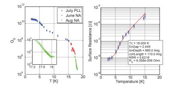
Figure 6: Q vs T measured with phase lock loop (PLL) or with network analyzer (NA) with weak coupling such that the  $Q_0{\sim}Q_L$  (left);  $R_s$  vs T from PLL data and polymorphic BCS fit (right).
