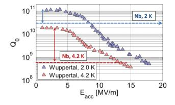
Figure 1: Q vs E curves at 2 K and 4.2 K for one of the best Nb<sub>3</sub>Sn cavities produced by U. Wuppertal [2]. The approximate values for a Nb cavity are shown for comparison.
