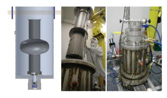
Figure 2: Cross-section of coating chamber (left), coating chamber being lowered into furnace (center), and UHV furnace with chamber inside (right).
