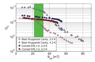
Figure 7: Q vs B curves of the Cornell and Wuppertal cavities. In green is the Cornell cavity's  $B_{c1}=27\pm5$  mT, which the cavity clearly exceeds without any indication of vortex dissipation.
