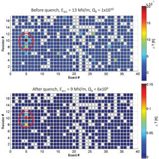
Figure 5: Temperature maps (which show the heating of the outer cavity surface relative to the helium bath) before quench, close to the quench field (top) and after the first quench (bottom). The region of strong localized heating is circled. Notice the difference in scale between the top and bottom.
