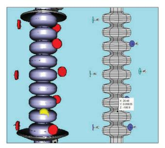
Figure 2: Quench position calculated with CS (left) and VPC (right) algorithms in the "strewn sensors" configuration. The yellow sphere on the left picture represents the uncertainty in quench position calculation.
