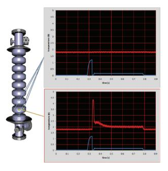
Figure 4: Sensor configuration with corresponding sensor temperature responses (red lines). Blue line is cavity transmitted RF power.
