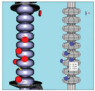
Figure 3: Quench position calculated with CS (left) and VPC (right) algorithms in the "concentrated sensors" configuration.
