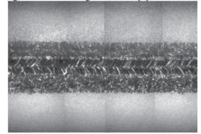
Figure 5: Optical image of cell 2 equatorial region after 800 °C treatment.
