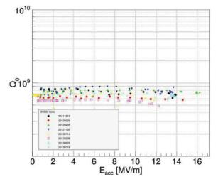
Figure 1: Cavity 3HZ02 Q0 vs. E<sub>acc</sub> for several RF tests. A flat low  $Q_0$  and its sharp drop indicate a possible poor surface condition or material inclusion.
