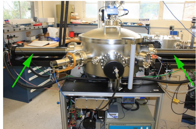
Figure 7: LBNL dual magnetron HiPIMS deposition chamber dedicated to the coating of 1.3 GHz cavities with niobium [27].
