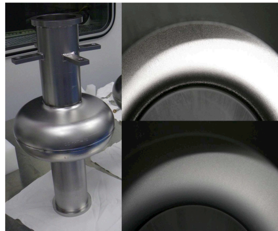
Figure 8: Coated cavity (left); view looking down into cavity before (top right) and after coating (bottom right).
