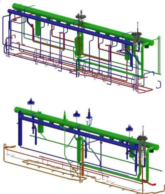
Figure 9: FRIB Beta=0.085 cryogenic systems (below) is greatly simplified when compared to the ReA6 cryogenic systems (above).
