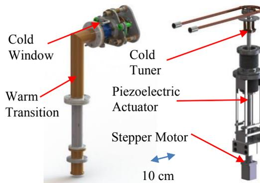
Figure 5: Quarter-wave power coupler assembly and warm transition by ANL (left). Tuner drive by FRIB (right).
