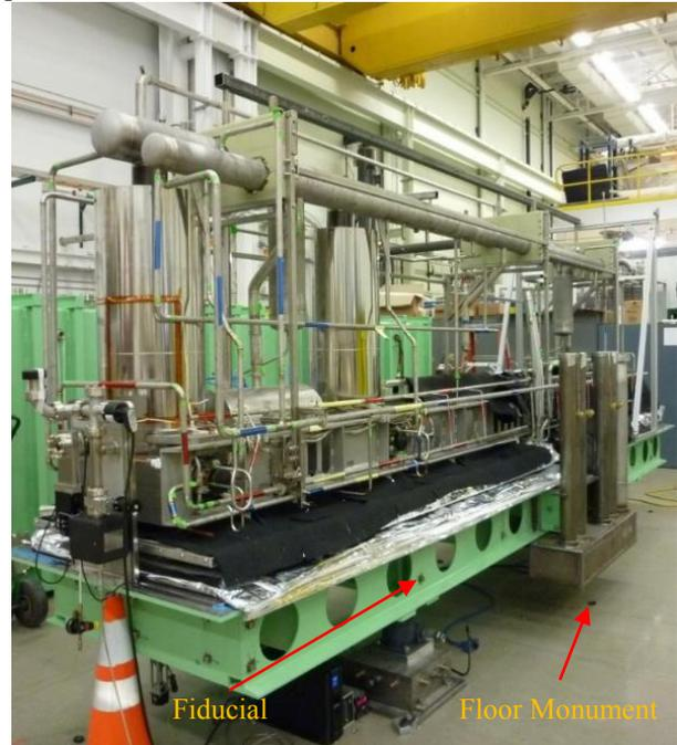
Figure 8: ReA6 cryomodule build with local network established to support alignment measurements.
