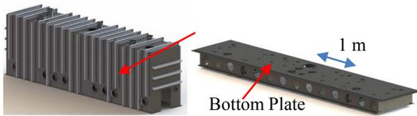
Figure 7: Vacuum vessel components. Vacuum vessel lid (left) is lowered onto bottom plate (right) and sealed by an EPDM O-ring.
