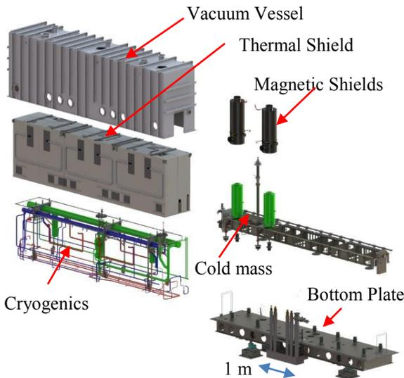
Figure 3: Sub-System of FRIB cryomodule design. Supported off the bottom plate is the cold mass system, where the resonators are protected by local magnetic shielding (right). The cryogenic system attaches to the cold mass. All assemblies are encapsulated by the thermal shield and vacuum vessel (left).
