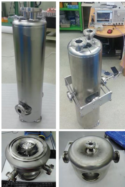
Figure 5: Photographs of prototype superconducting cavities [QWR(top left), HWR(top right), SSR1(bottom right), SSR2(bottom left)].
