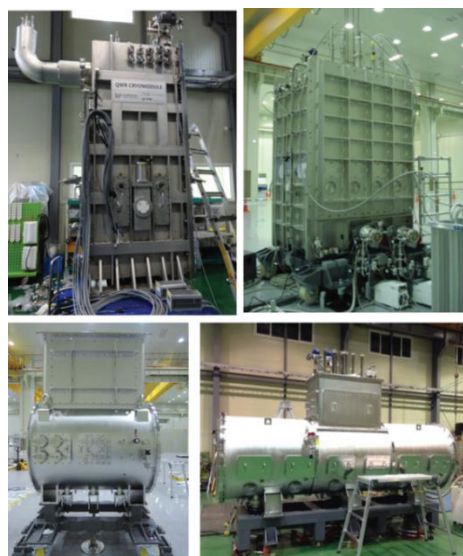
Figure 10: Photos of prototype cryomodules fabricated through domestic vendors.
