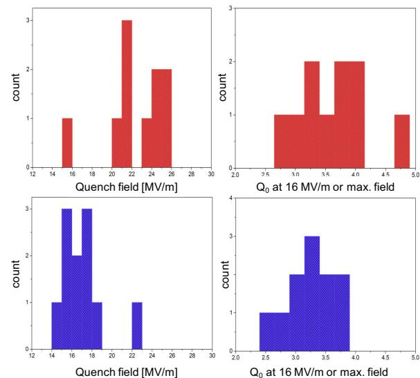
Figure 1: Top: 2K nine-cell cavity performance values using the "2N6A" nitrogen doping recipe. Average quench field: 22.2 MV/m. Average  $Q_0$ :  $3.6 \times 10^{10}$ . Bottom: 2K nine-cell cavity performance values using the "20N30A" nitrogen doping recipe. Average quench field: 16.3 MV/m. Average  $Q_0$ :  $3.2 \times 10^{10}$ .
