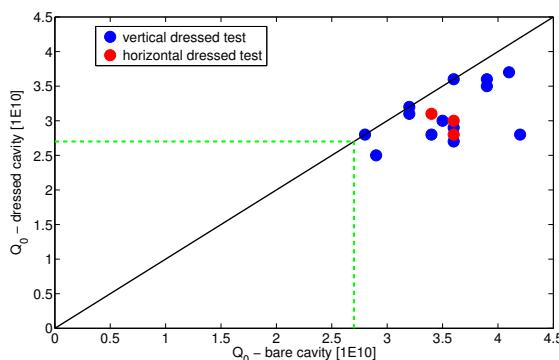
Figure 5: Comparisons of 2K  $Q_0$  at 16 MV/m in horizontal test before and after LHe tank welding ("dressing").  $Q_0$  values are corrected for cavity flange losses during performance testing, which will not be present in LCLS-II cryomodule installation.
