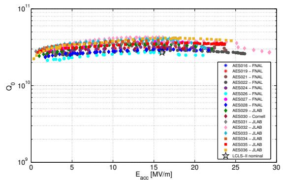
Figure 3: 2K  $Q_0$  vs  $E_{acc}$  performance of bare N-doped cavities in vertical test.  $Q_0$  values are corrected for cavity flange losses during performance testing, which will not be present in LCLS-II cryomodule installation.
