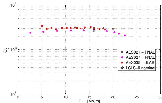
Figure 6: 2K  $Q_0$  vs  $E_{acc}$  performance of dressed N-doped cavities in horizontal test.
