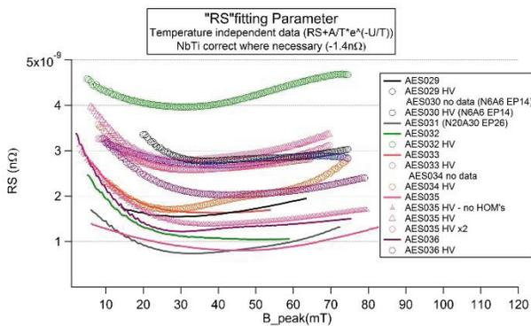
Figure 3: Temperature independent fitting parameter "RS" extracted from the Q vs. Eacc vs. T data before (solid lines) and after (open circles) cavity dressing.
