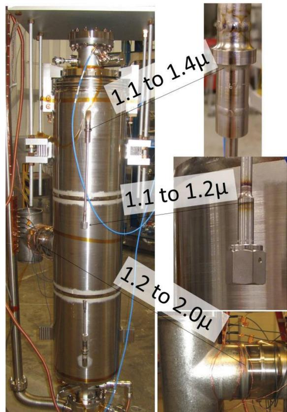
Figure 4: Left 9 cell cavity in helium vessel ready for vertical test showing permeable components on helium vessel (welds and exploded bonded joints) and their surveyed permeability range and locations on right.
