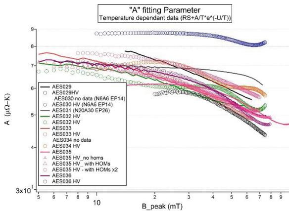
Figure 2: Temperature dependant fitting parameter "A" extracted from the Q vs. Eacc vs. T data, before (solid lines) and after (open circles) cavity dressing.
