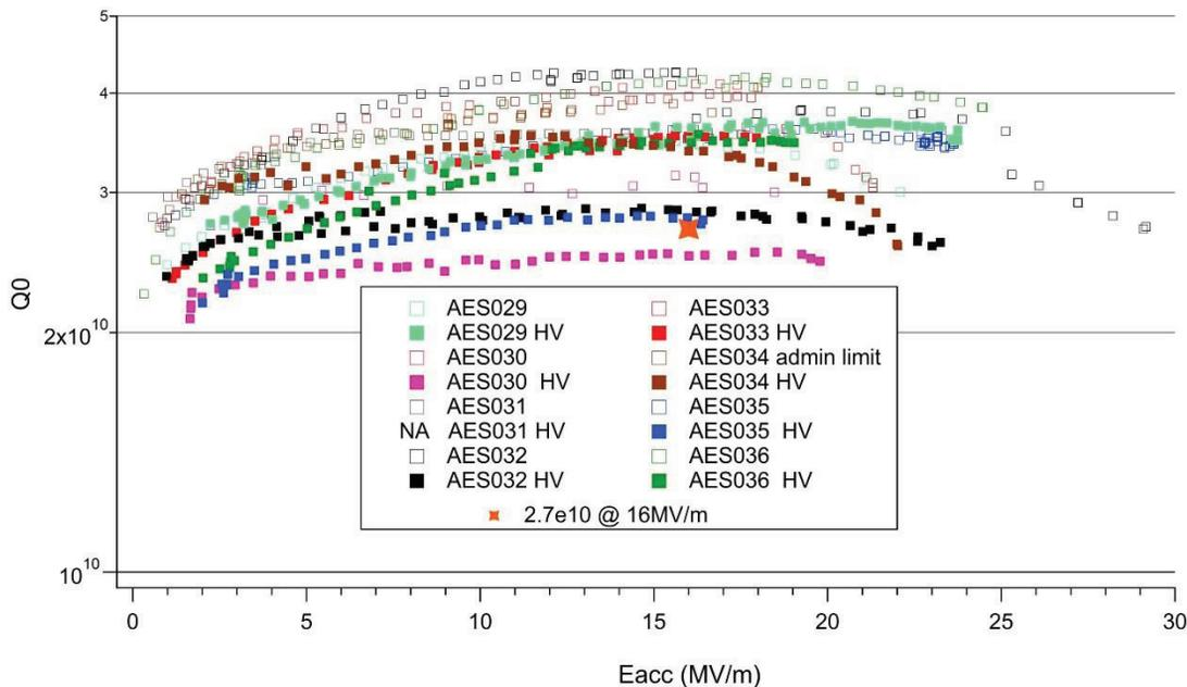
Figure 1: Q vs Eacc @ 2.0K before (solid squares) or after (open squares) HV welding and HOM installation. All data corrected to superconducting glanges if SS flanges were used.
