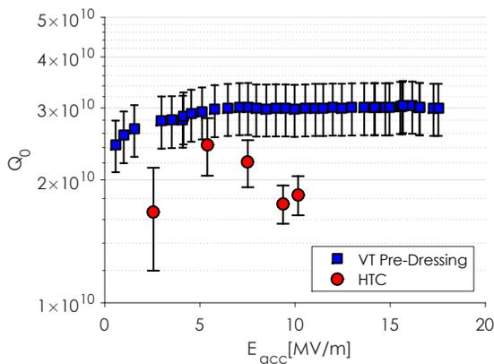
Figure 4:  $Q_0$  vs  $E$  performance at 2.0 K before and after assembly in the HTC for HTC9-5 (ACC031).
