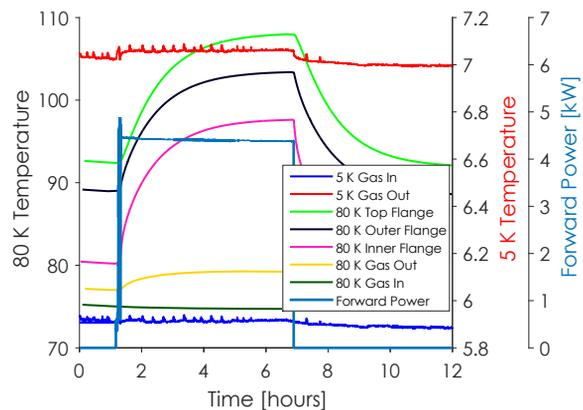
Figure 6: Plot of coupler heating on the 5 K and 80 K system. Note that the coupler in the HTC was cooled with 5 and 80 K gas whereas LCLS-II will use thermal straps to cool the couplers.
