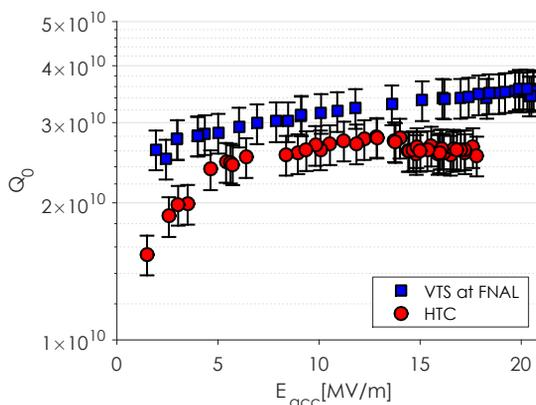
Figure 2:  $Q_0$  vs E performance at 2.0 K before and after assembly in the HTC for HTC9-2 (AES011).
