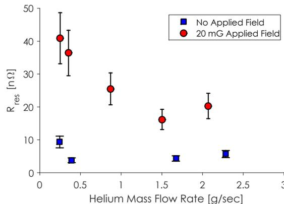
Figure 9: Residual resistance vs helium mass flow rate in an applied external magnetic field of 20 mG and no external magnetic field. Larger mass flow rate resulted in less residual resistance due to more efficient flux expulsion.
