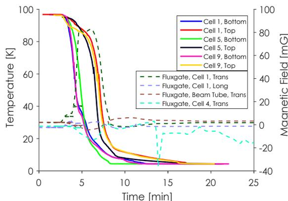
Figure 8: A typical cool down for the LCLS-II helium vessel.
