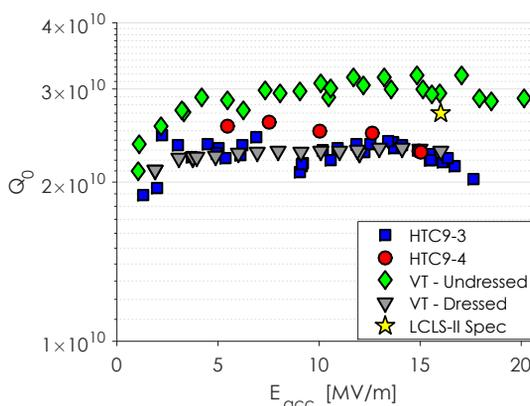
Figure 3:  $Q_0$  vs E performance at 2.0 K before and after assembly in the HTC for HTC9-3 and HTC9-4 (AES018).
