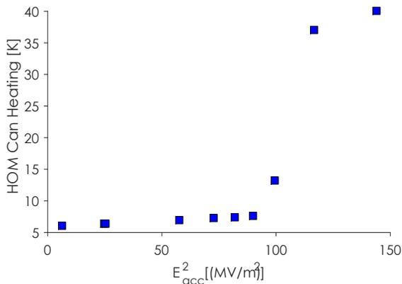
Figure 7: Heating on the HOM can during HTC9-5. This is a clear symptom of multipacting. The highest point was not in steady state since temperatures got too high and the power was administratively turned off.
