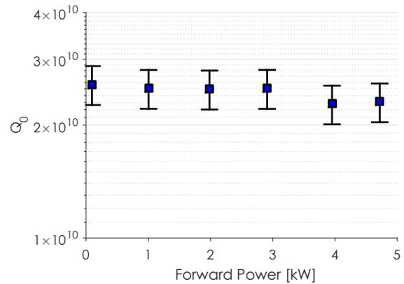
Figure 5:  $Q_0$  at 10 MV/m vs forward power during HTC9-4.  $Q_0$  was unaffected up to 3 kW after which it slightly dropped.
