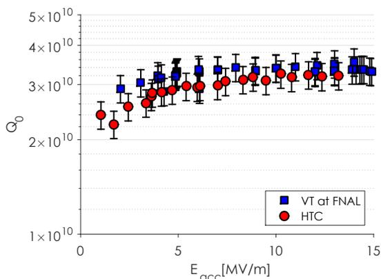
Figure 1:  $Q_0$  vs E performance at 2.0 K before and after assembly in the HTC for HTC9-1 (ACC012).
