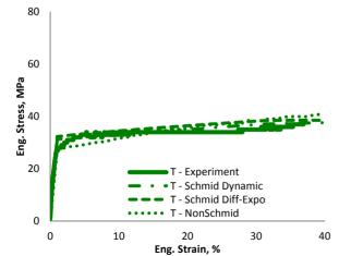
Figure 3: Sample T was used to calibrate the Dynamic hardening and the non-Schmid models, simultaneously with sample P. This figure also shows the prediction of the Differential-Exponential model for sample T.
