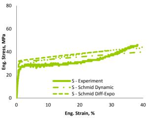
Figure 6: Comparing predictions of the models with the experiment of S. Predictions of the Dynamic hardening and non-Schmid models are close. The Differential-Exponential model predicts single slip behavior for this sample.
