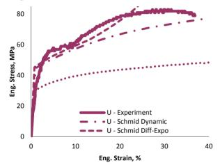
Figure 7: Comparing predictions of the models with the experiment of U. Prediction of the Dynamic hardening model is close to the experiment. The non-Schmid model fail for this sample. The Differential-Exponential model predicts a two-stage behavior for this sample.
