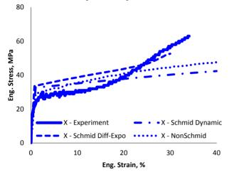
Figure 10: Comparing predictions of the models with the experiment of X. Predictions of the Dynamic hardening and non-Schmid models are close. The Differential-Exponential model predicts a two-stage behavior for this sample.
