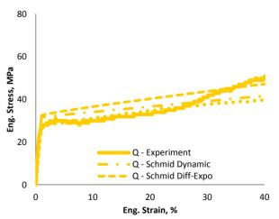
Figure 5: Comparing predictions of the models with the experiment of Q. Predictions of the Dynamic hardening and non-Schmid models are close. The Differential-Exponential model predicts single slip behavior for this sample.
