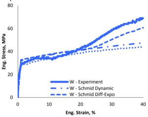
Figure 9: Comparing predictions of the models with the experiment of W. Predictions of the Dynamic hardening and non-Schmid models are close. The Differential-Exponential model predicts a two-stage behavior for this sample.
