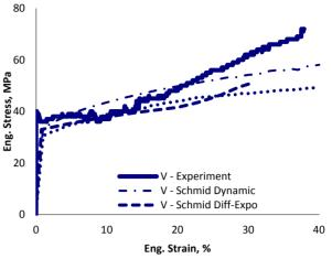
Figure 8: Comparing predictions of the models with the experiment of V. Predictions of the Dynamic hardening and non-Schmid models are close. The Differential-Exponential model predicts a two-stage behavior for this sample.
