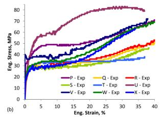
Figure 1: (a) The tensile axis of samples used in this study. (b) Stress-strain response of annealed single crystal samples.
