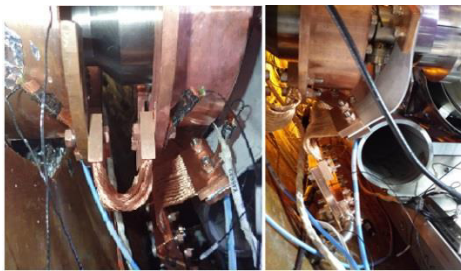
Figure 4: Coupler thermal 70K (left) and 5K connection.
