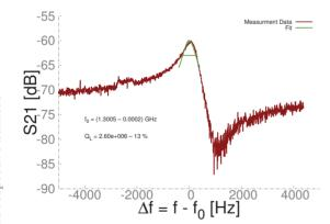
Figure 4: Fitting a Lorentz-curve to the resonance signal of the TM010- $\pi$  mode reveals the  $Q_L$ .
