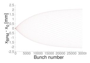
Figure 8: Simulated bunch position after the beam gets kicked by HOM in the ACM cryomodule.
