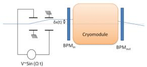
Figure 7: Potential setup for beam based HOM measurements. A pair of RF deflectors creates a modulation in the beam offset to the beam axis and excites a HOM if the modulation frequency matches to a HOM.
