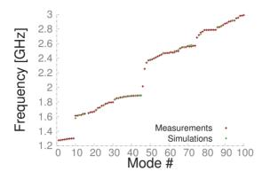
Figure 3: HOM frequencies measured on the ICM.
